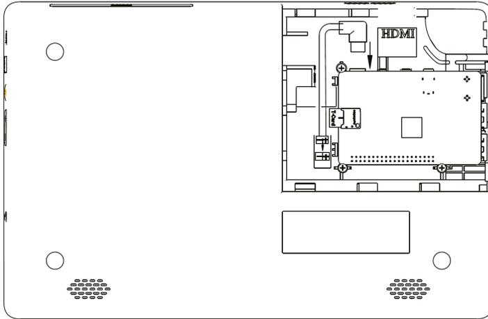
**6.** Then take the USB camera cable and connect it to one of the USB ports of your Raspberry Pi.
