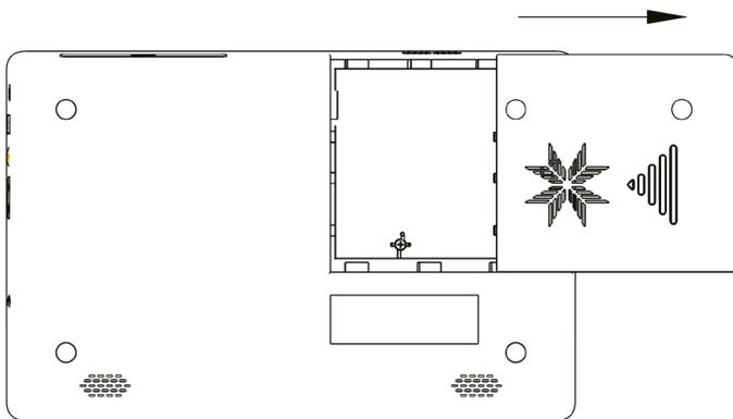
3. Insert the Raspberry Pi into the mounting tray. Then insert the screws to secure your Raspberry Pi.
