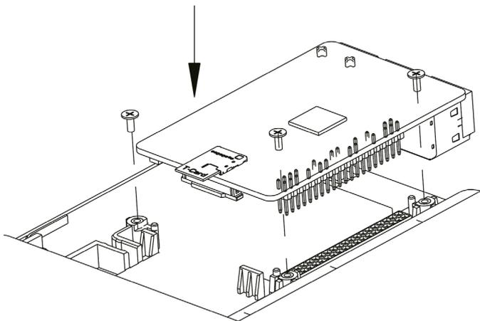
4. Connect the micro-HDMI adapter board to the HDMI port of your Raspberry Pi.
